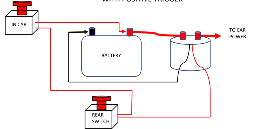
IN CAR AND REAR SHUT OFF SYSTEM WITH POSITIVE TRIGGER USING OPTIONAL SAFETY SWITCH ON GROUND SIDE
