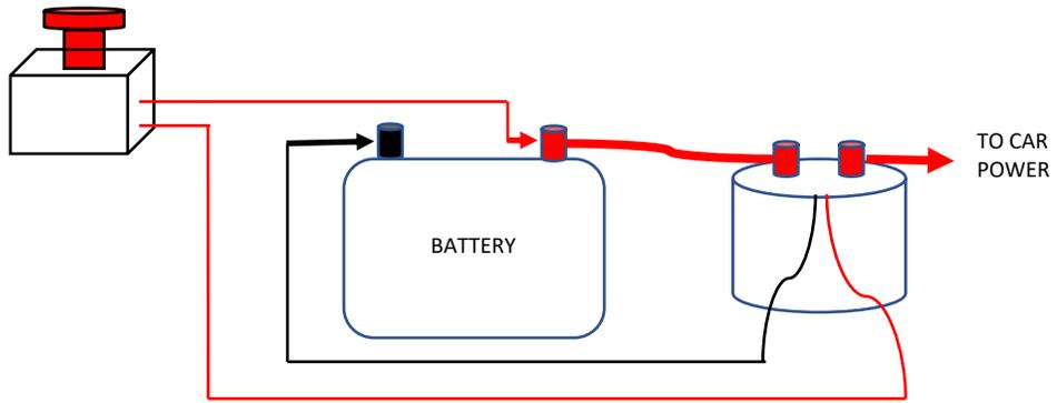
IN CAR AND REAR SHUT OFF SYSTEM WITH POSITIVE TRIGGER
