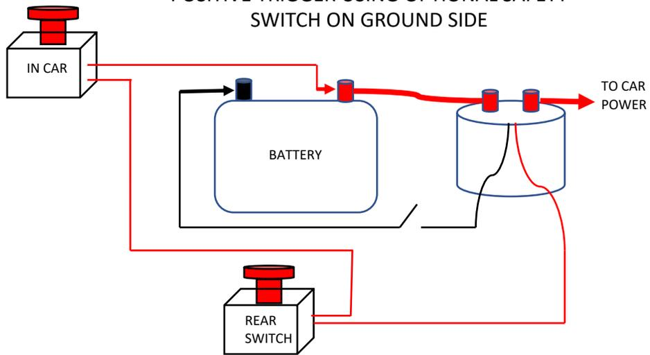
IN CAR AND REAR SHUT OFF USING BOTH TRIGGER METHOD ONE FOR EACH SWITCH
