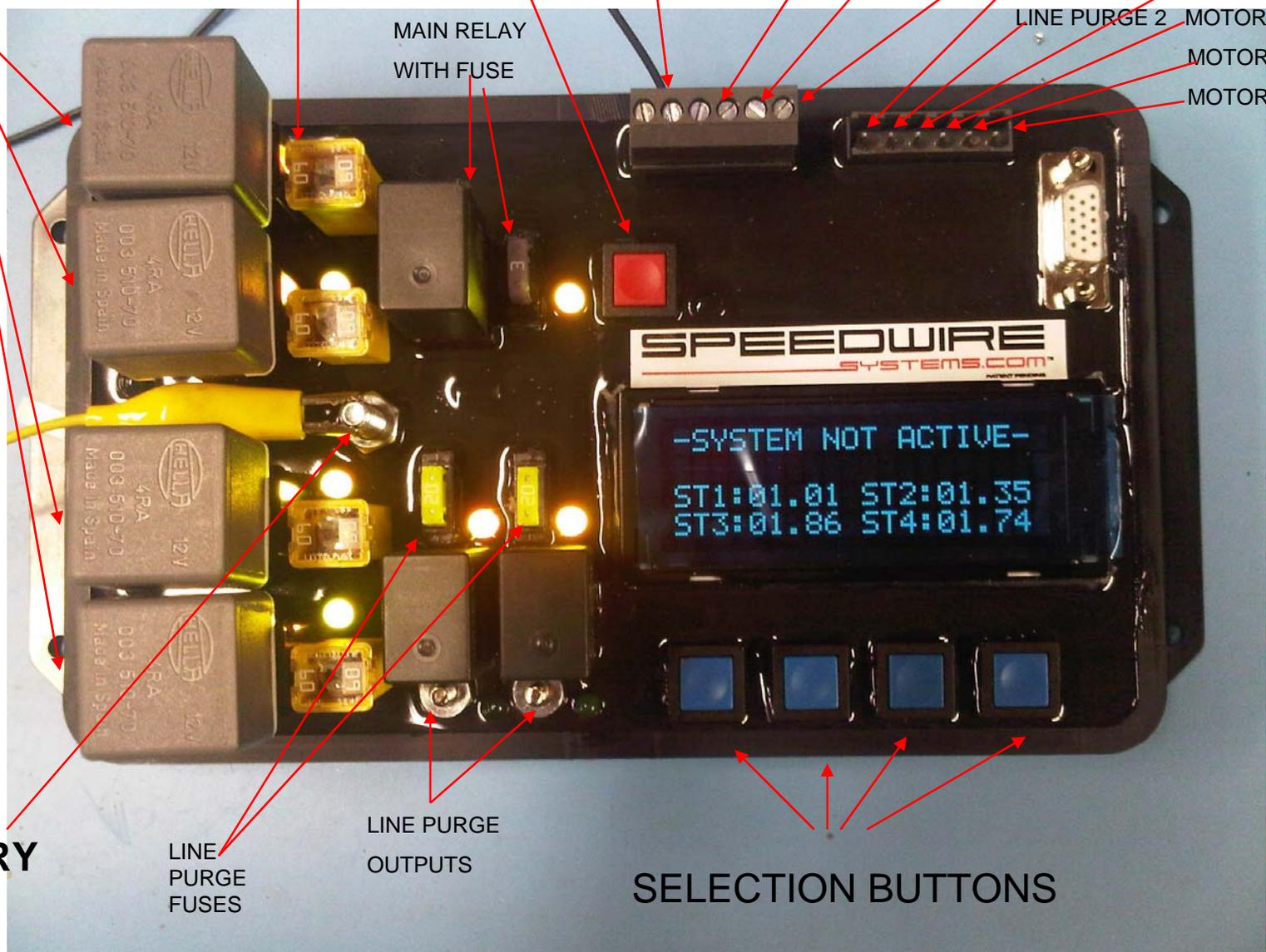
THIS IS AN EXAMPLE OF USING A CLUTCH SWITCH APPLICATION AND **WITHOUT DATA CABLE FROM SWITCH PANEL** TO NITROUS CONTROLLER, IF USING THIS METHOD YOU WILL NOT BE USING T-12 AND T-13 CIRCUITS ON MAIN BOARD, THE INTERRUPT FUNCTION IS DONE THROUGH THE NITROUS CONTROLLER.
