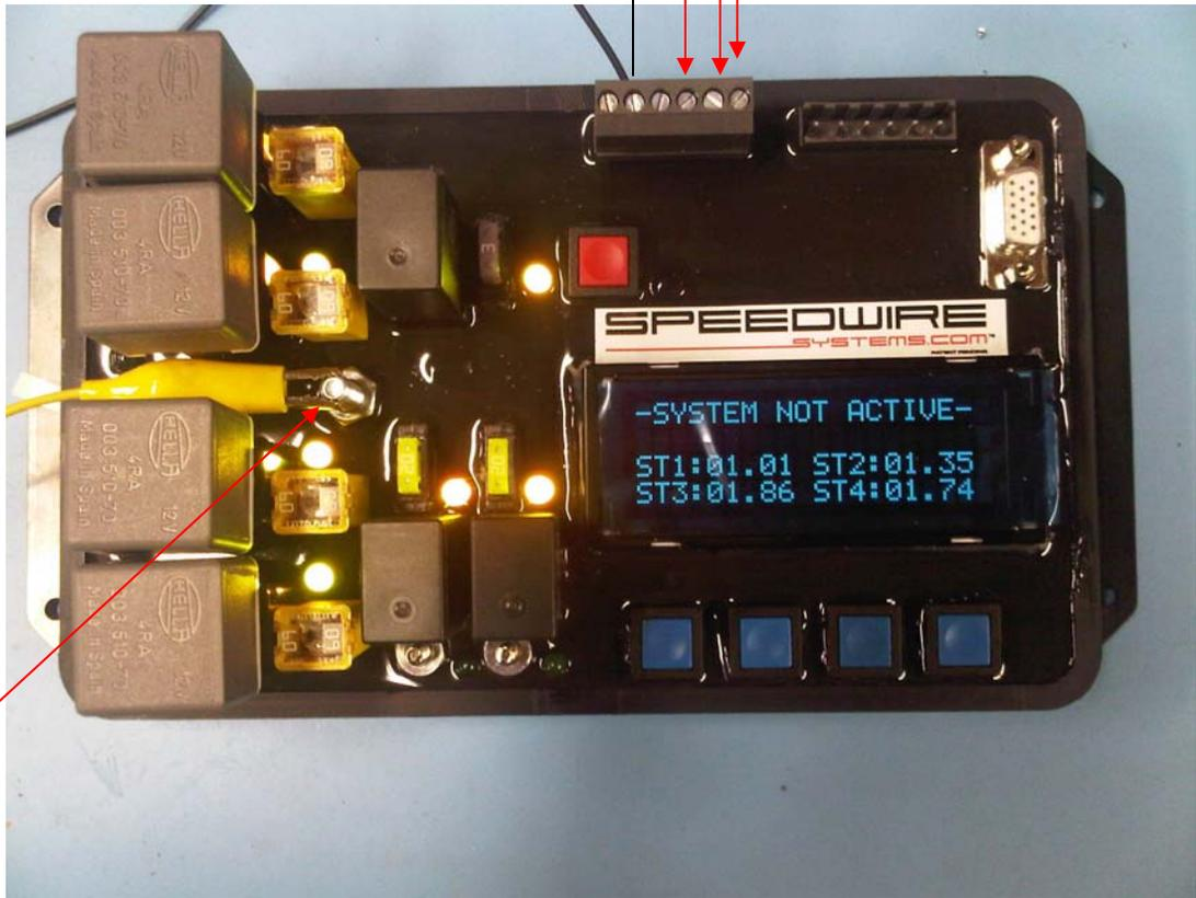
MAIN POWER 6 GAUGE WITH 4 SYSTEMS 8 GAUGE WITH 2 SYSTEMS
