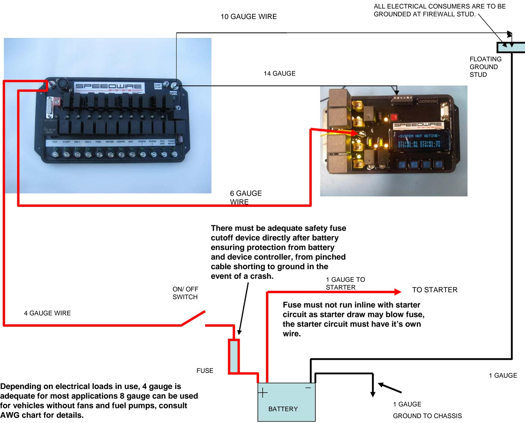
There must be adequate safety fuse cutoff device directly after battery ensuring protection from battery and device controller, from pinched cable shorting to ground in the event of a crash.
